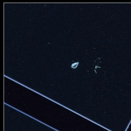
Particle on semiconductor wafer (Darkfield)
